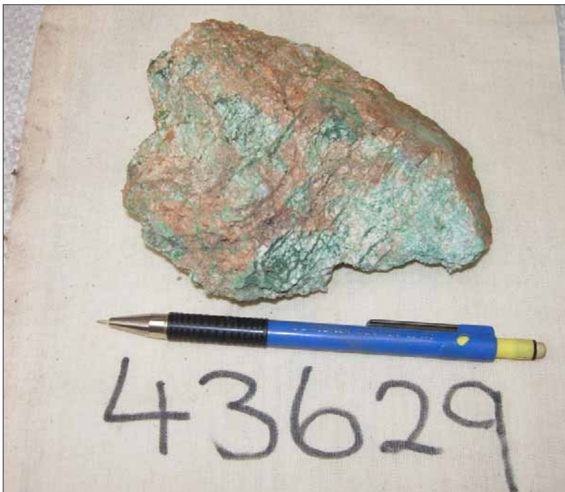
Plate 3 Sample 43629, assaying 14.9% copper, is from the granodiorite near the base of the hill, suggesting possible depth to the mineralisation
