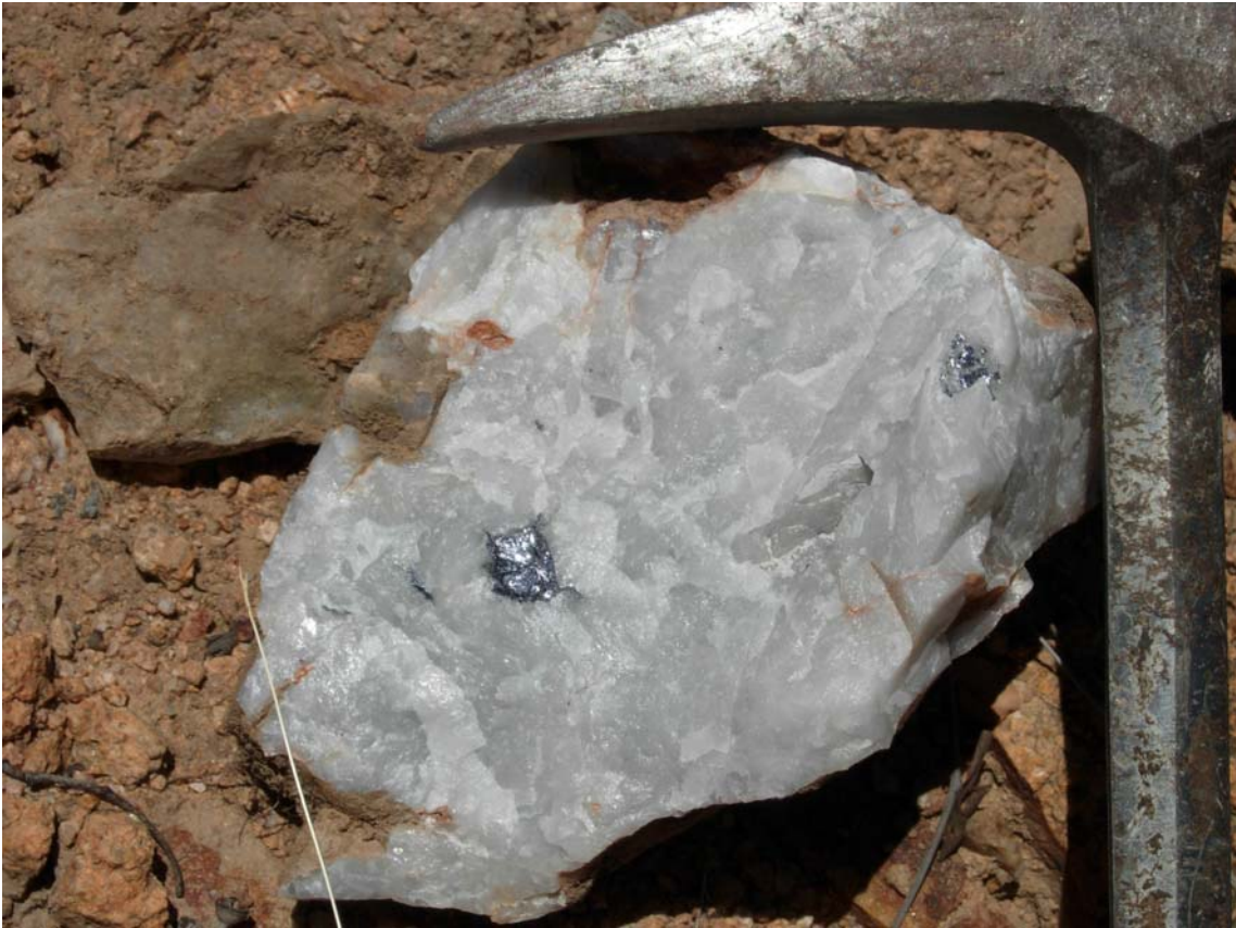
Plate 3: Visible molybdenum within quartz vein (Site 3).
