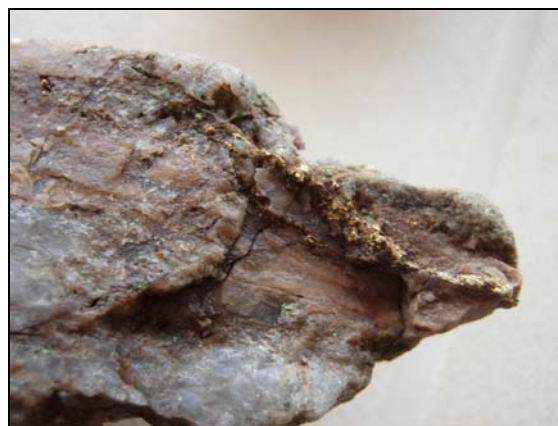
Plate 3: Gold within quartz from Percy West Lease Sample supplied by A Zabel, Leaseholder
