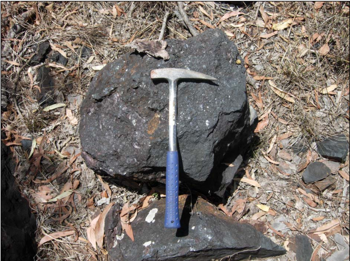
Plate 2: Iron from near site 3 on Figure 1. Massive crystalline magnetite
