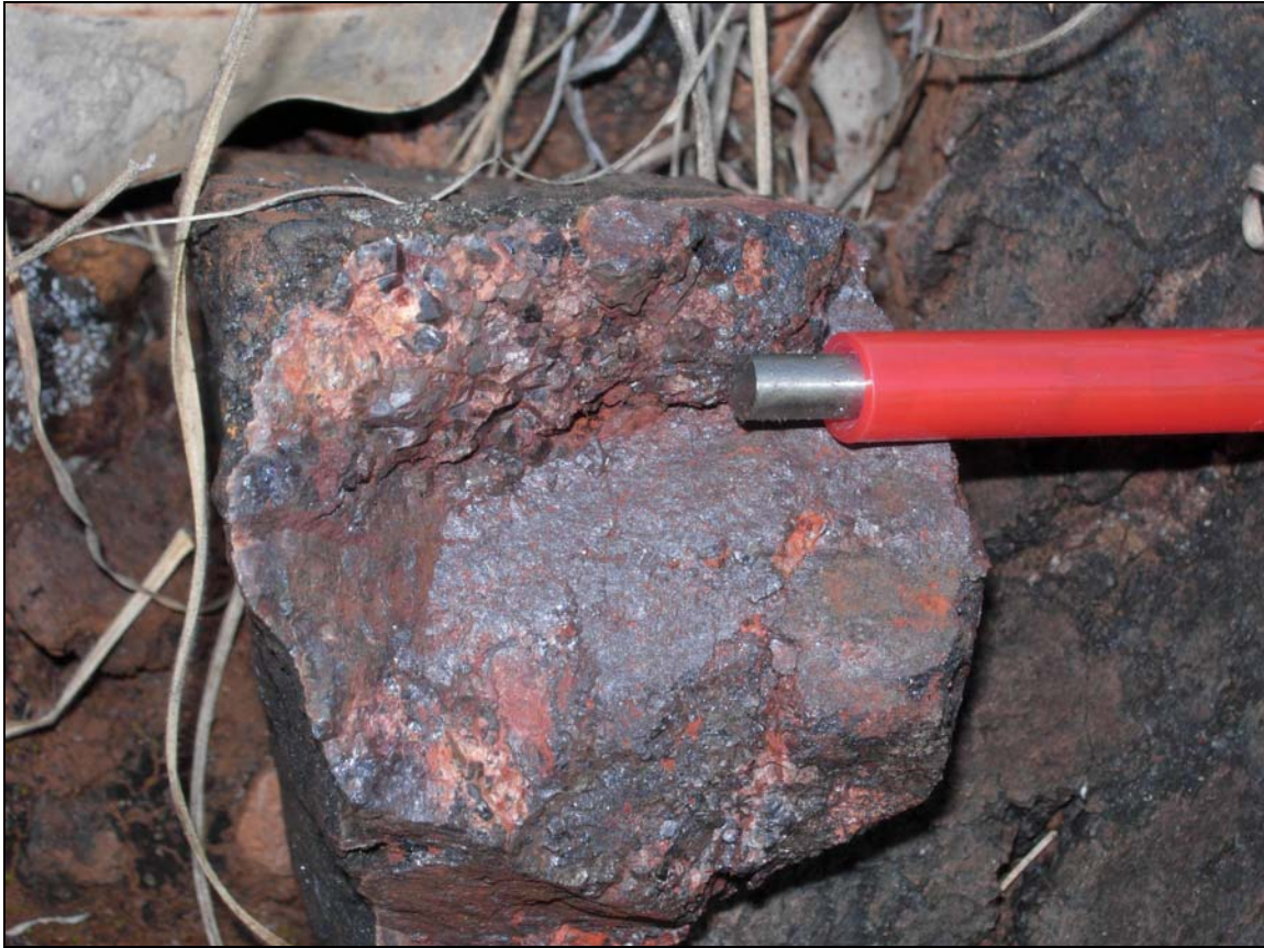
Plate 1: Coarse magnetite crystals with minor hematite produced by weathering of primary magnetite (rock assayed 68.7% Fe)
