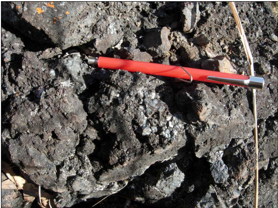
Plate 2: Coarse magnetite crystals (assay 65.1% Fe)
