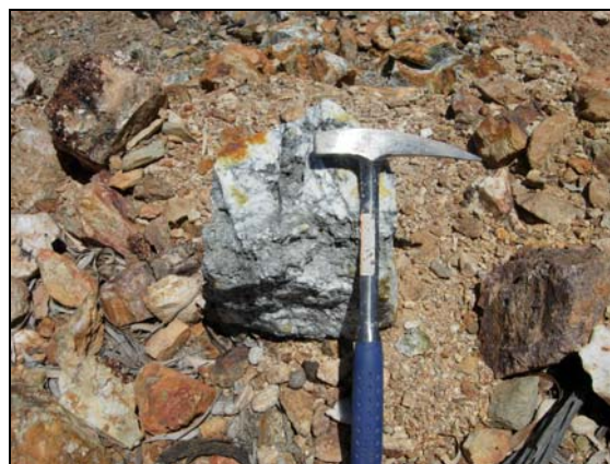
Plate 2: Sample of sulphide-rich quartz which hosts gold from Canadian Lease
