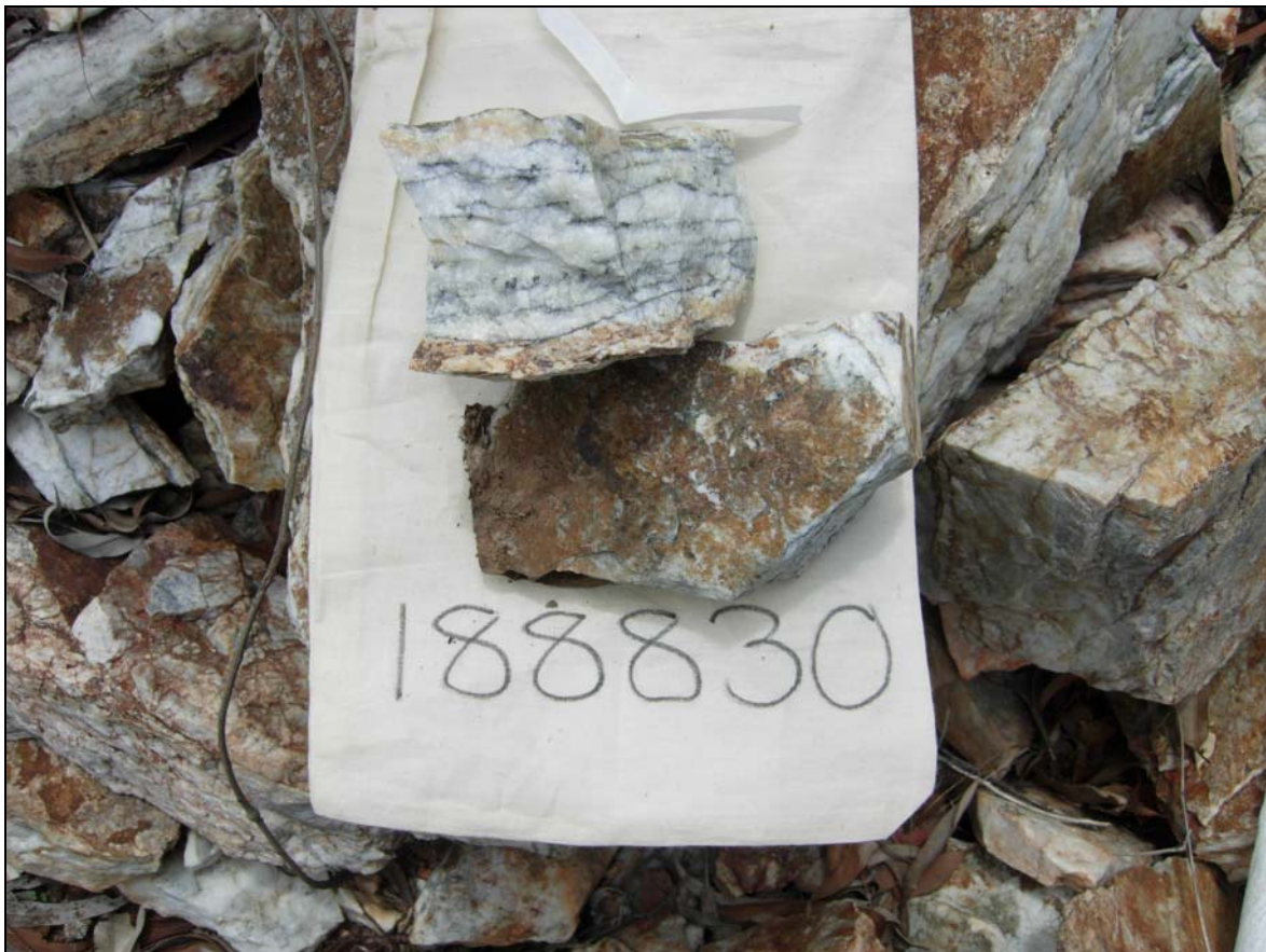
Plate 2: Sample 188830 – quartz with sulphide veins – assayed 43.5 g/t gold
