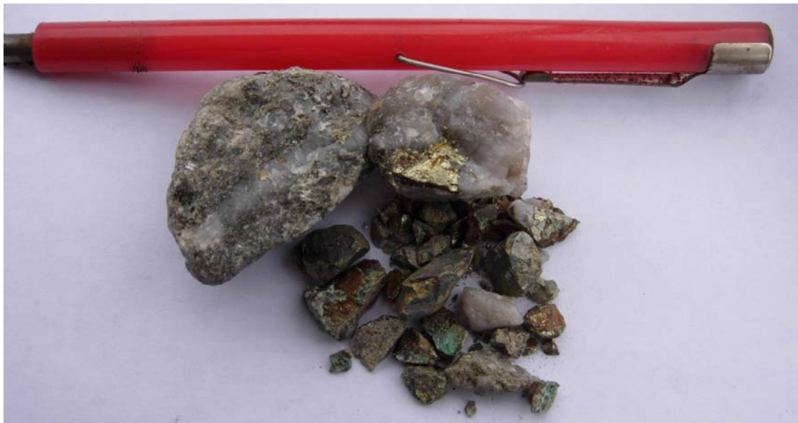
Plate 1: Chalcopyrite rich drill chips from 99-100m within drill hole URC002 (assay result 1 m @ 10.9 g/t Au)
